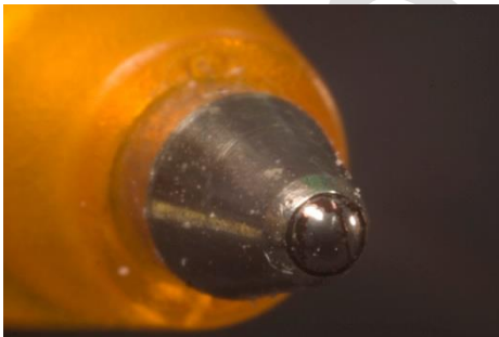
Figure 2: Close Up of Ballpoint Pen Tip
