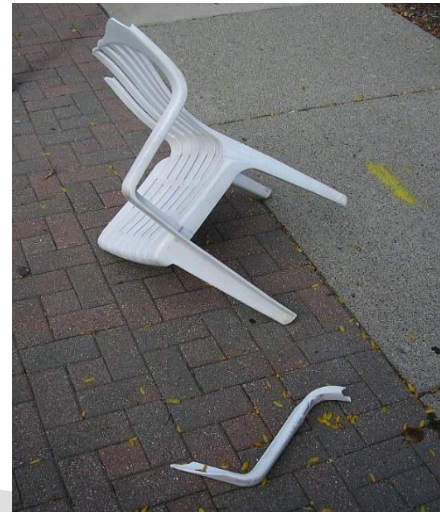
Figure 5: Plastic Chair with Broken Leg
